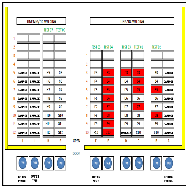
Figure 1 LEV's Mapping Plan and Performance Evaluation
