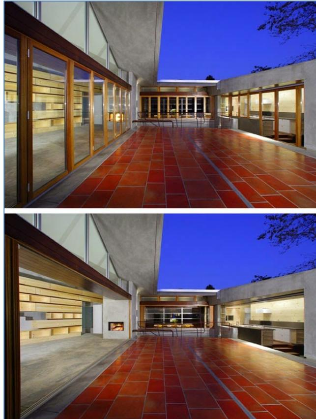
**Figure 3: Bifold glass wall system to regulate comfort**
