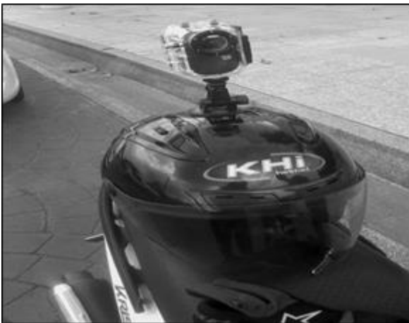
Fig. 3 The SJ1000 camera was equipped on the experimental helmet
