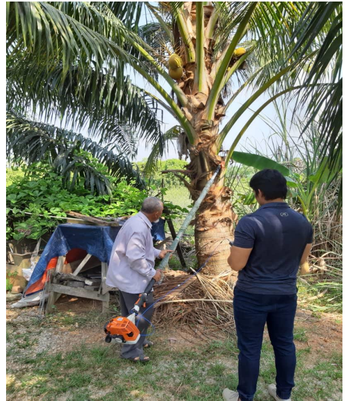
Fig. 3 Measurement of vibration using HVM 100 with tri-accelerometer attached to the Cantas machine
