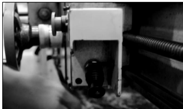
Fig. 5 Switch for spindle rotation of Lathe
