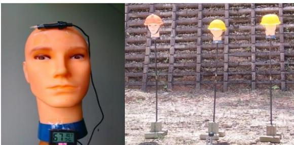
Fig. 1 Head Manikin with temperature probe and display (Left); Experimental set up (Right)
