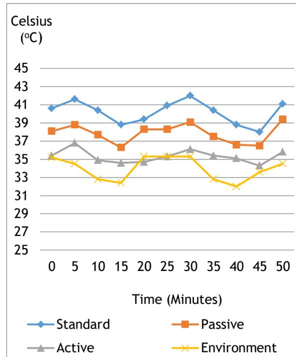
**Fig. 3 Temperature against time for a different type of safety helmet and the environmental temperature**
