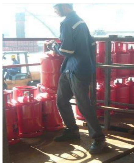
**Fig. 2 Activity 2: Rolling LPG cylinder onto the platform**
