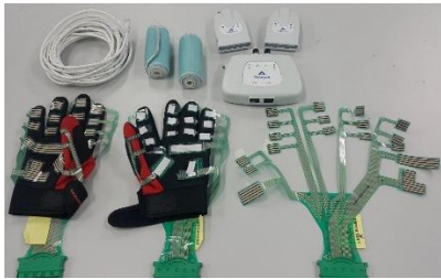
Figure 2 Tekscan tactile grip force and pressure measurement (Grip system).
